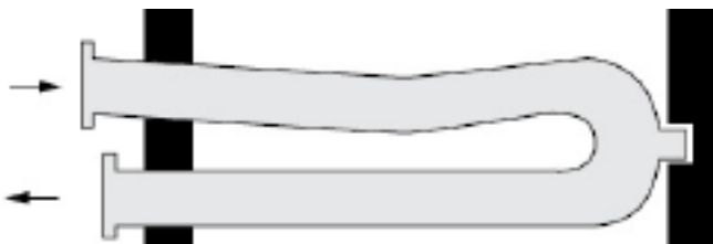
Typical tube sagging/bending of the firing leg.
