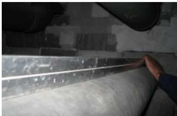
After 1.5 years of service in the hottest zone of a furnace, the W-tube with the burner leg made of Kanthal® APMT showed a sagging of 0–2 mm (0–0.1 in).
