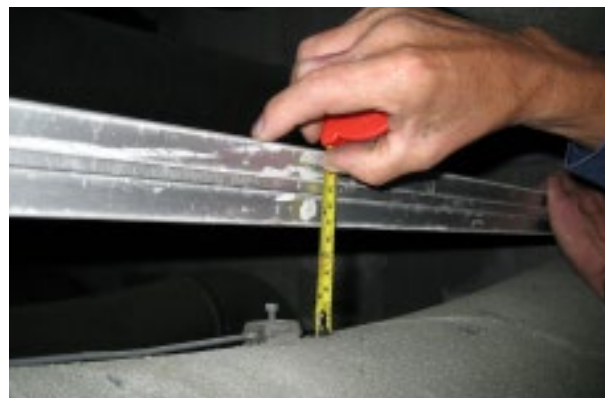
The reference tubes, made of conventional cast material (iron-nickel-chromium), had sagged 55–65 mm (2.2–2.6 in). Two of the reference tubes were replaced after only 1.5 years.
