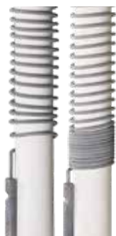
Comparison between Kanthal APM (left) and conventional FeCrAl (right) after 1250 h at max 1225°C element temperature.
